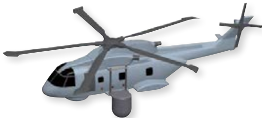
Thales is proposing to repackage and migrate the Cerberus tactical suite and Searchwater 2000AEW radar into the Merlin HM2 as the basis for the Crowsnest role fit. (Image: Thales)
