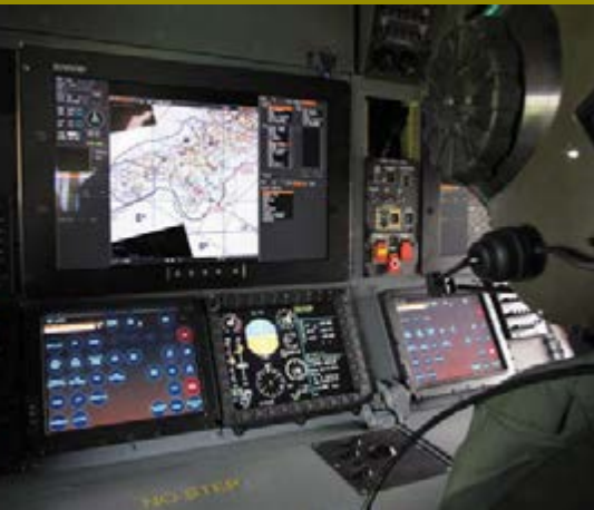
The Vigilance suite reuses the mission system now in service on the Merlin HM2. Lockheed Martin believes this significantly de-risks its Crowsnest bid. (Photo: author)
